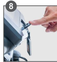
8 Start machine by pushing the key
