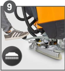
9 Lower brush unit by using the manual lever (by foot) or automatically by pressing the button
