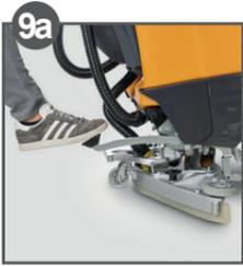
9a Lower brush units by using the manual lever (by foot)
